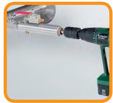
Drilling under pressure
